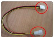
Sub-power cable for SATA Converter board
